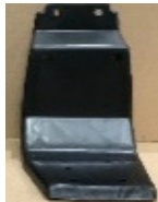
Recycled Carbon Fibre ("RCF") RB Brackets
