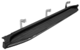
Blow Molded Running Boards
