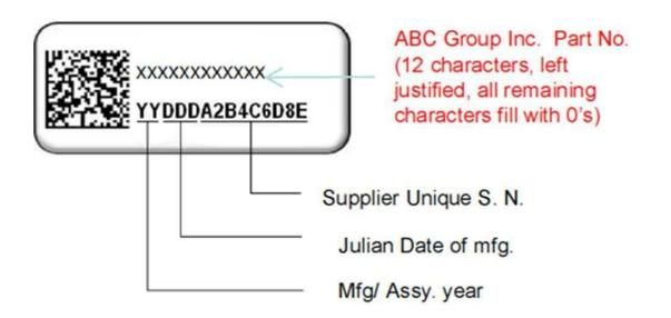
Standardized 2D Bar code format (QR or Data matrix) across all components and internal assemblies.
