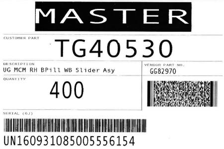
All products received by ABC must contain a serial number that is clearly identified on each label and every container. Suppliers can add date codes etc. within their allotted space.
